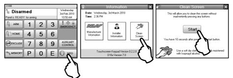
Step 4. The touch screen will be disabled for 10 seconds. Clean the bare screen or the protective film using a soft dry cloth or a cloth moistened with Isopropyl Alcohol.
